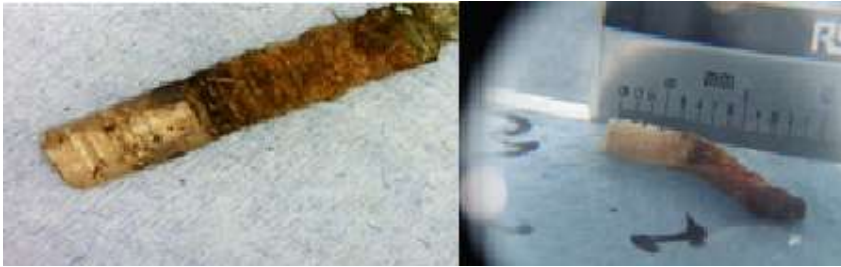
Fig.1 To show typical mini cores. Left image: Approx. one third (circa 3-4mm) xylem tissue. Right image: Distortion and cylindrical asymmetry during drying process
