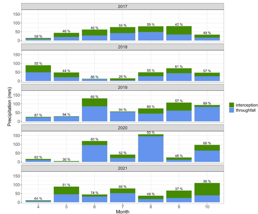
Figure S 15: Local monthly precipitation, shown as stacked throughfall ( P_r mm) and interception ( P_i mm), at BIFoR FACE for treatment seasons 2017 to 2021. Percentage throughfall is indicated above each combined bar.
