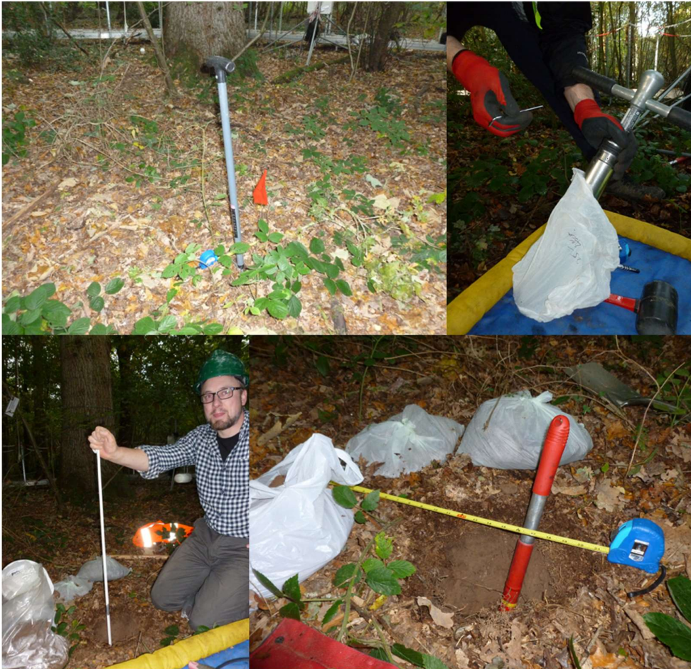
Figure 2- 5: Photos of soil temperature installation near to an oak in a typical array.
