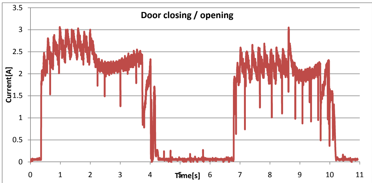
Figure 5-10. Current sense for door closing / opening with doubled PWM duty cycle changes.
