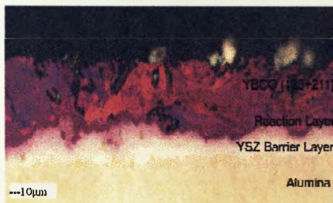
Figure 5.5.4 Polarised light micrograph of the YBCO/YSZ/ \text{Al}_2\text{O}_3 structure. The major phases existent are shown. Supplied by Watcham et al. [5.5.1].
