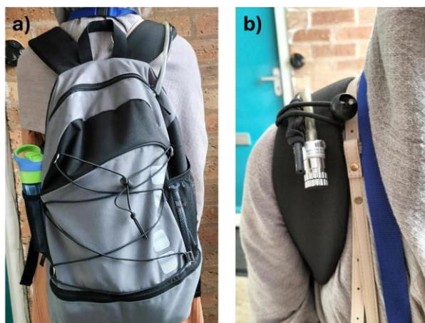
Figure 7. Sampling setup (a) shows a backpack carried personal exposure devices, (b) shows the position of inlet within the breathing zone of a researcher.
