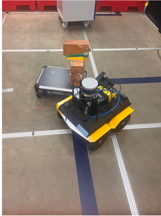
Figure 5.20: Real-world experiment showing the robot reaching the estimated source location
