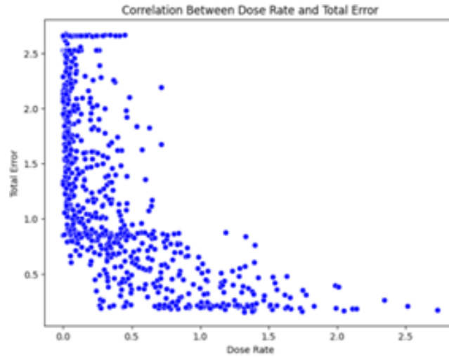
Figure 5.13: Correlation between Dose Rate and Total Error for Path 2. A negative correlation is observed: as the dose rate ( \mu\text{Sv/h} ) decreases, the total error (m) increases.
