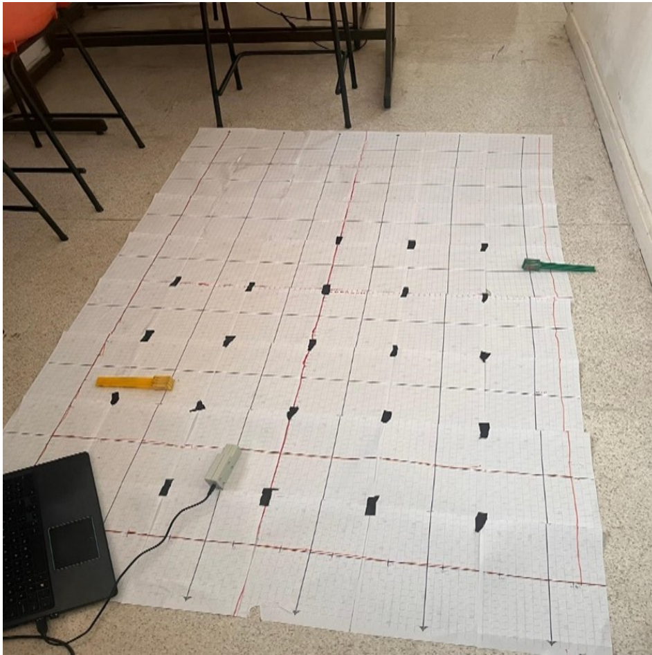
Figure 5.44: Measurement system designed to determine the position of multiple radiation sources.
