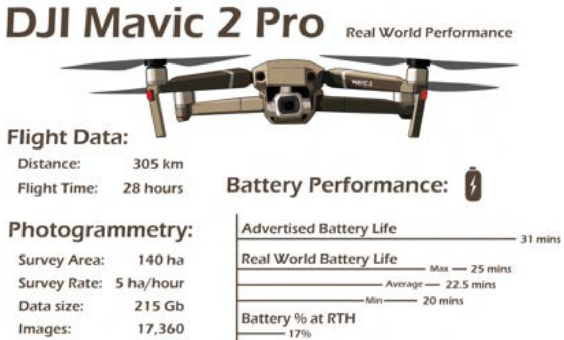
Figure A.1: Real world drone performance. Data representative of 60 flights. RTH, Return To Home, an automated process by which the drone returns to its take-off location when on low battery.
