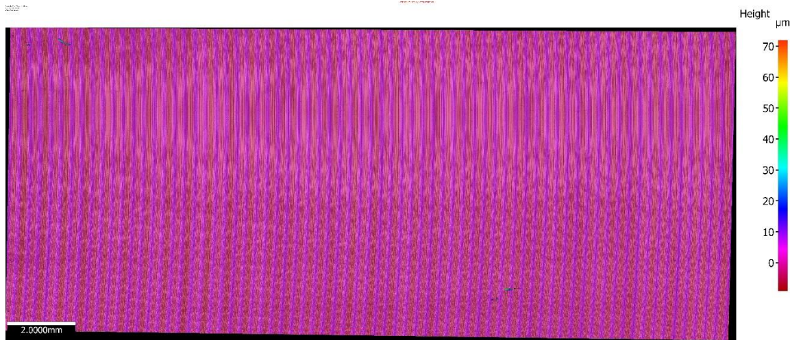
Figure 105 Surface area scan of the 3.2 \mu\text{m} vertical milling block.
