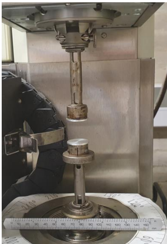
Figure 7 Parallel plate rheometer setup with 25 mm aluminium plates before adhesive application. The heat chamber, designed to wrap around the fixture columns, is not in position and is situated out of frame to the left.
