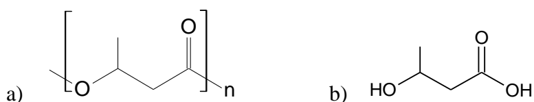
Figure 20: Structure of a) polyhydroxybutyrate (PHB, (C_4H_6O_2)_n ) and b) its monomer, hydroxybutyrate (HB, C_4H_6O_8 ).
