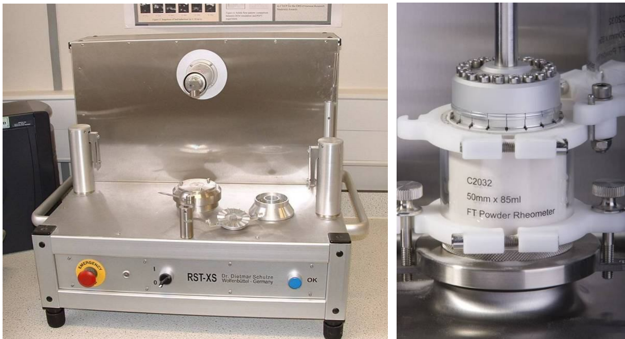
Figure 2.1: RST-XS and FT4 shear cells
