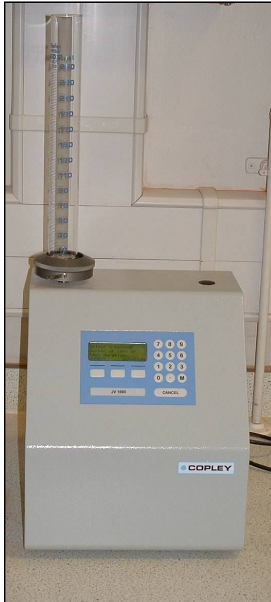
Figure 2.36: Single Vessel Jolting Volumeter
