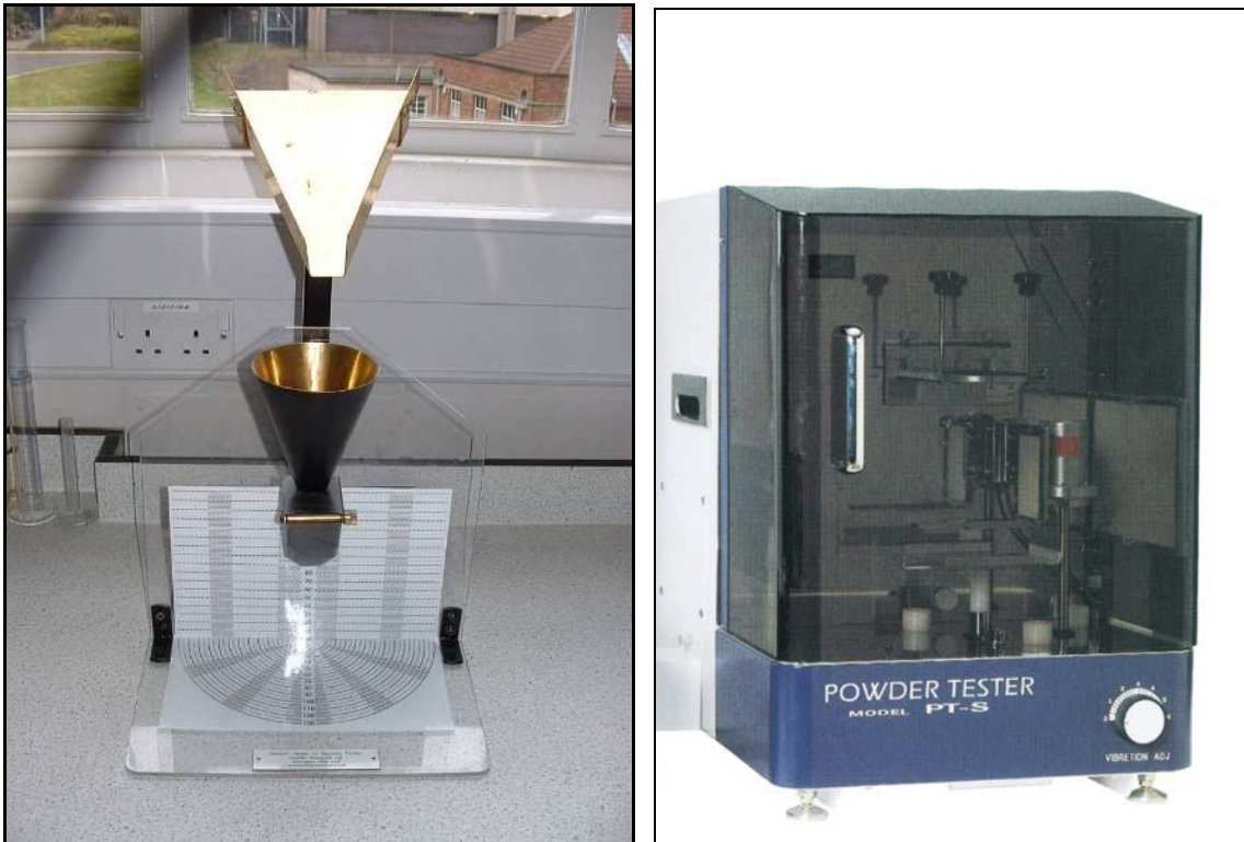
Figure 2.33: Geldart AOR tester (left) and Hosokawa Powder Tester – including an AOR test (right).
