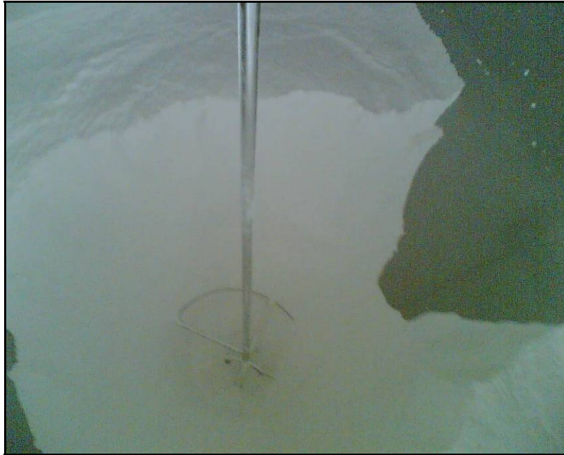
Figure 4.31: Rathole formed in IBC containing Avicel 102 during test of second sample
