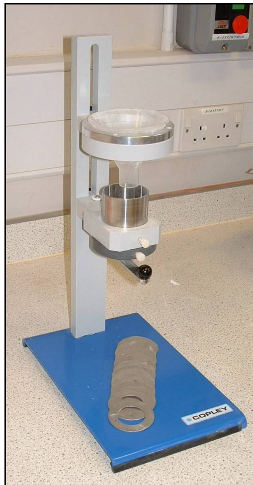
Figure 2.40: The Flowability Tester Model BEP2 Powder Flowability Tester
