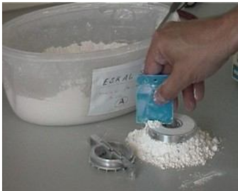
Figure 2.4: Filling of the RST-XS Shear Cell (reproduced from the Schulze web site http://www.dietmar-schulze.de )
