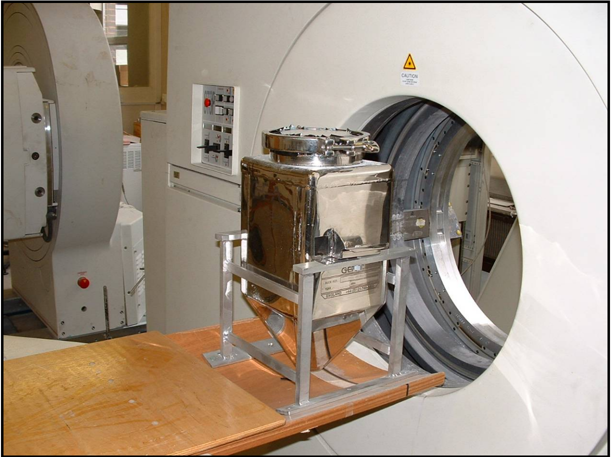
Figure 3.26: Mini-IBC located in its support frame prior to insertion into the measurement cavity inside the camera
