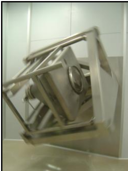
Figure 3.2: A tumble blender in operation
