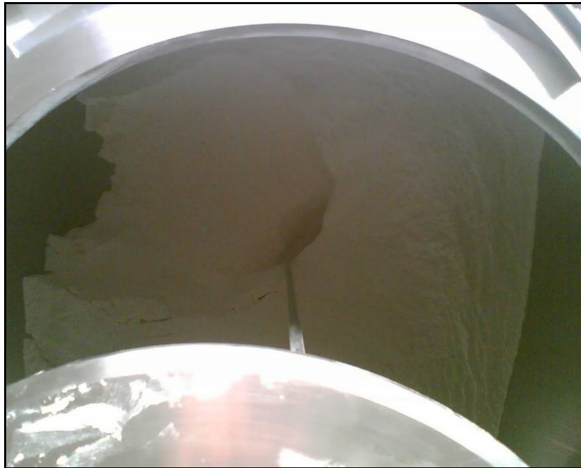
Figure 4.27: Rathole formed in IBC containing Avicel 102 during Test 2
