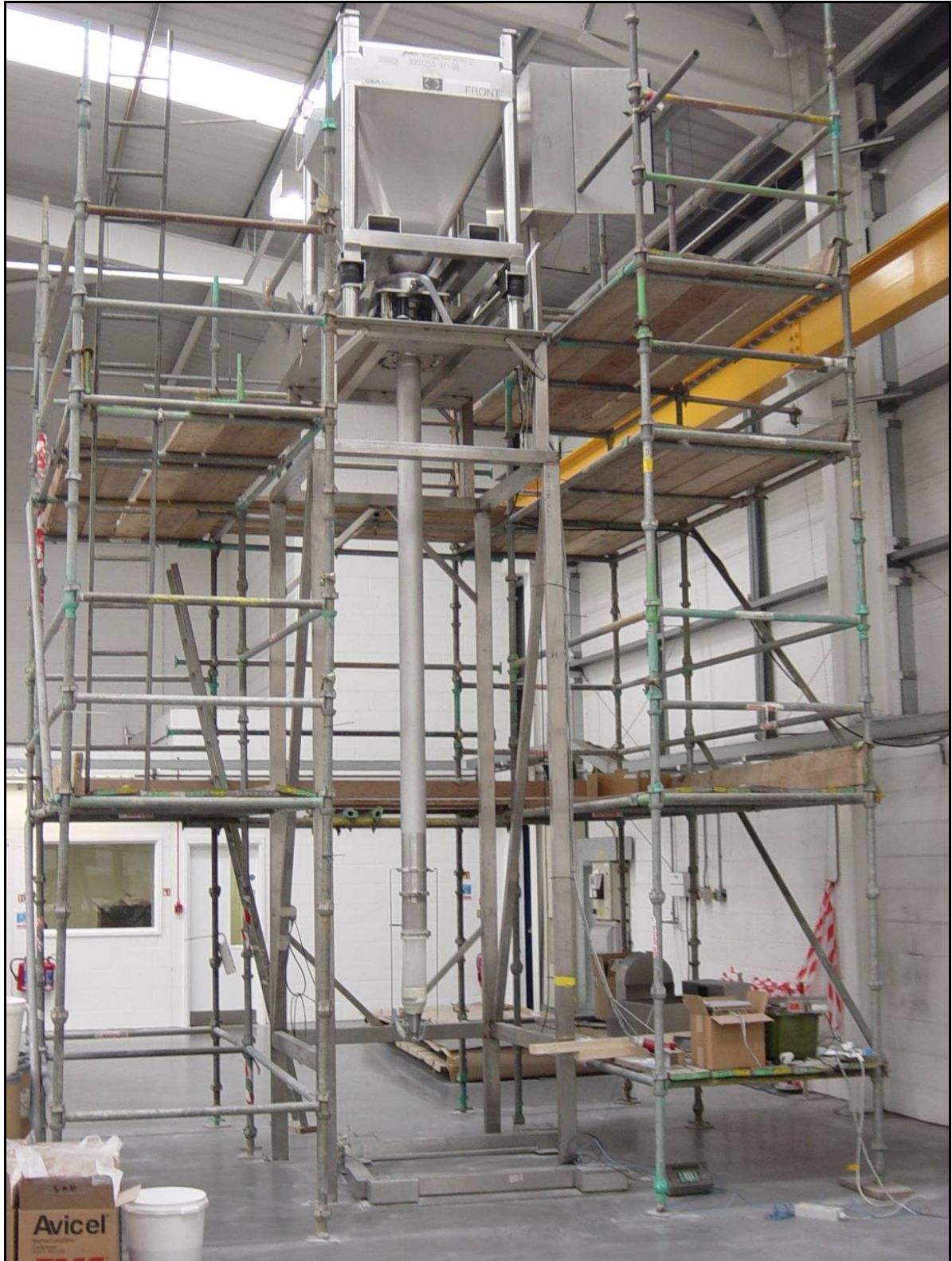
Figure 4.24: Discharge Station and Decel Tube with IBC containing the placebo located in position before operation with a load cell frame located under the discharge point to monitor the flow rate of the powder
