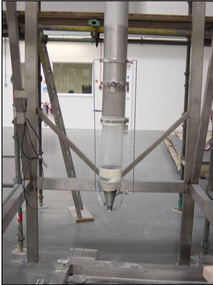
Figure 4.25: Detail of the discharge point of the Decel test rig
