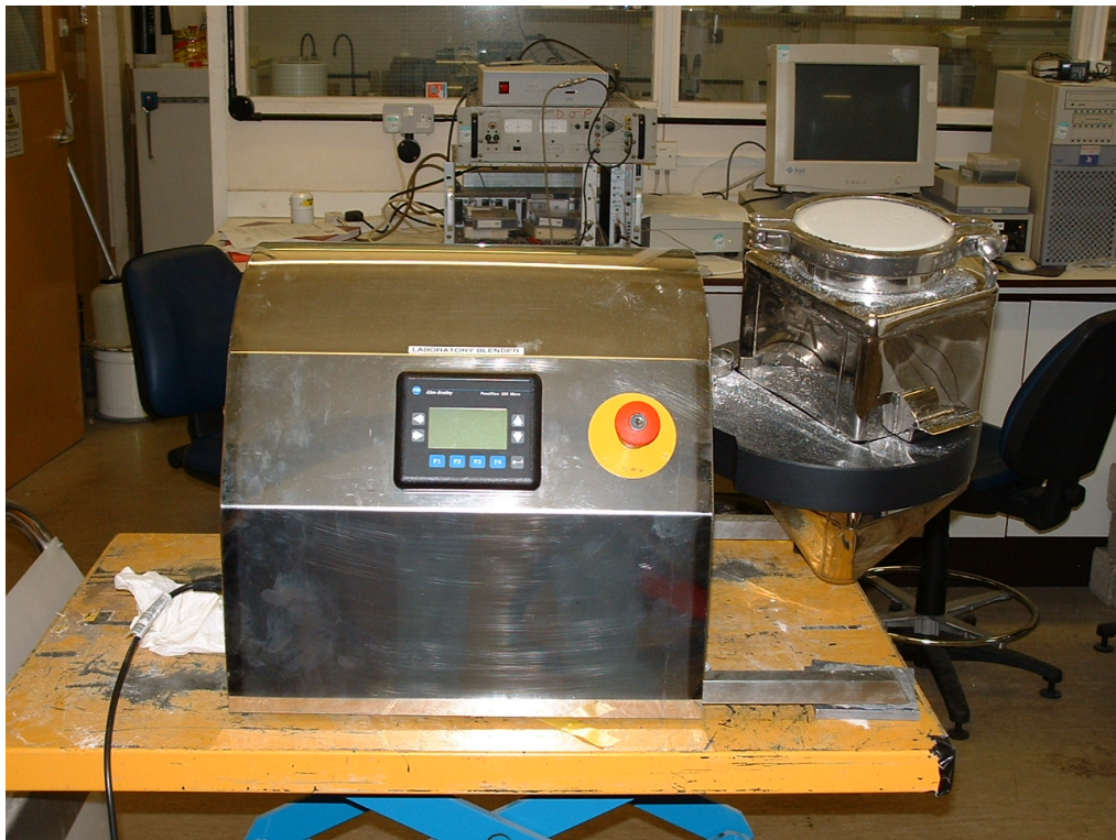
Figure 3.4: Laboratory Scale Blender in-situ prior to PET experiment
