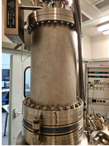
Figure 2.4 Cryogenic equipment of LT-STM. The \text{LN}_2 and LHe can be filled from the top.
