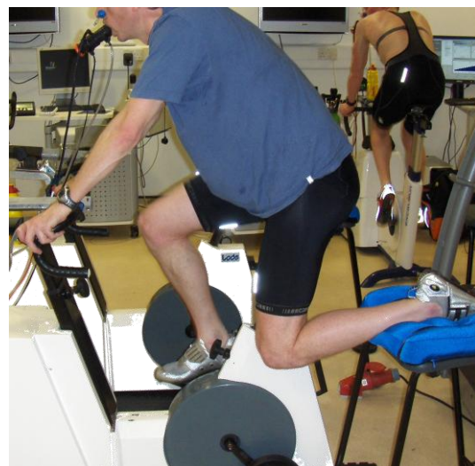
Figure 2.2: SL Subject completing a SL VO_{2max} test on the specifically modified Lode cycle ergometer, complete with contralateral counterweight device.
