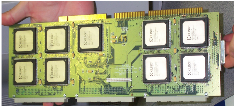
Figure 11 : HAL-15 Reconfigurable Computing Board with 10 Xilinx XC4062 chips (One FPGA located on the reverse side)[64]
