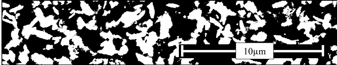
Figure 4-8 Converted black and white region of interest shown in Figure 4-7 used for volume fraction analysis of \text{TiB}_2 particles within the grain boundary material
