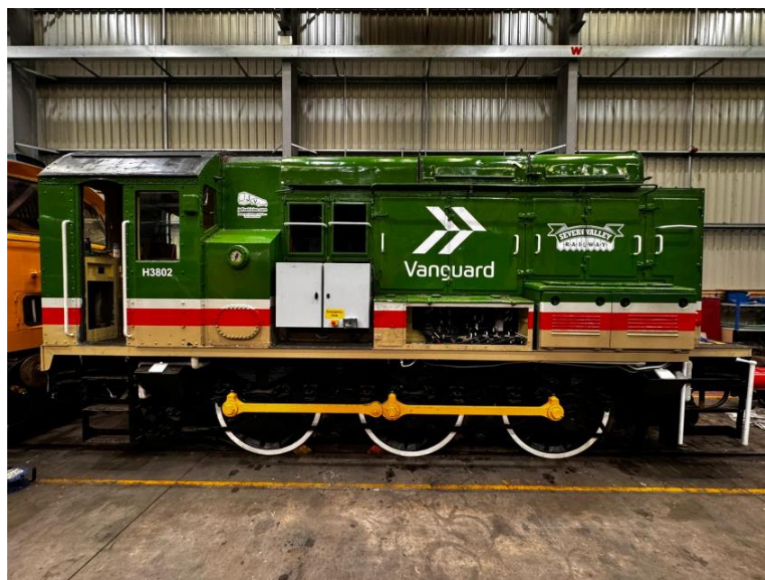
Figure 7.7: HydroShunter in development at the Severn Valley Railway, provided by Vanguard Sustainable Transport Solutions Limited, 2024
