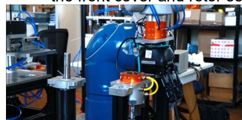
(h) Step 8: Staubli robot picks the electric gripper
