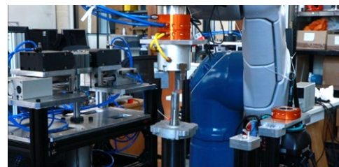
(f) Step 6: Staubli robot places the front cover and rotor set
