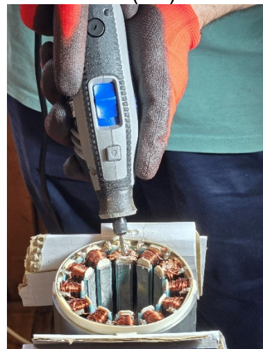
(f) Manual step 5: Coil disassembly
