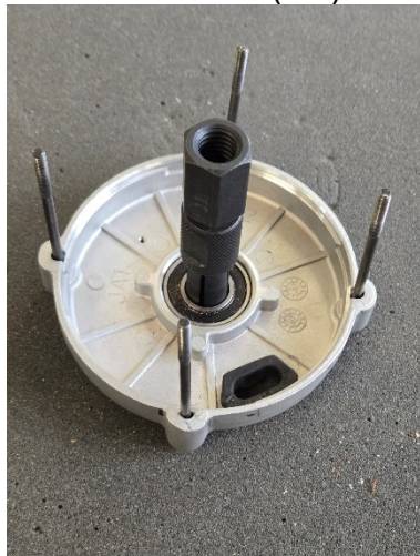
(c) Manual step 4: Press-in task (T.1) - A
