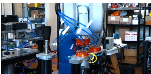
(g) Step 7: Staubli robot places the pneumatic gripper
