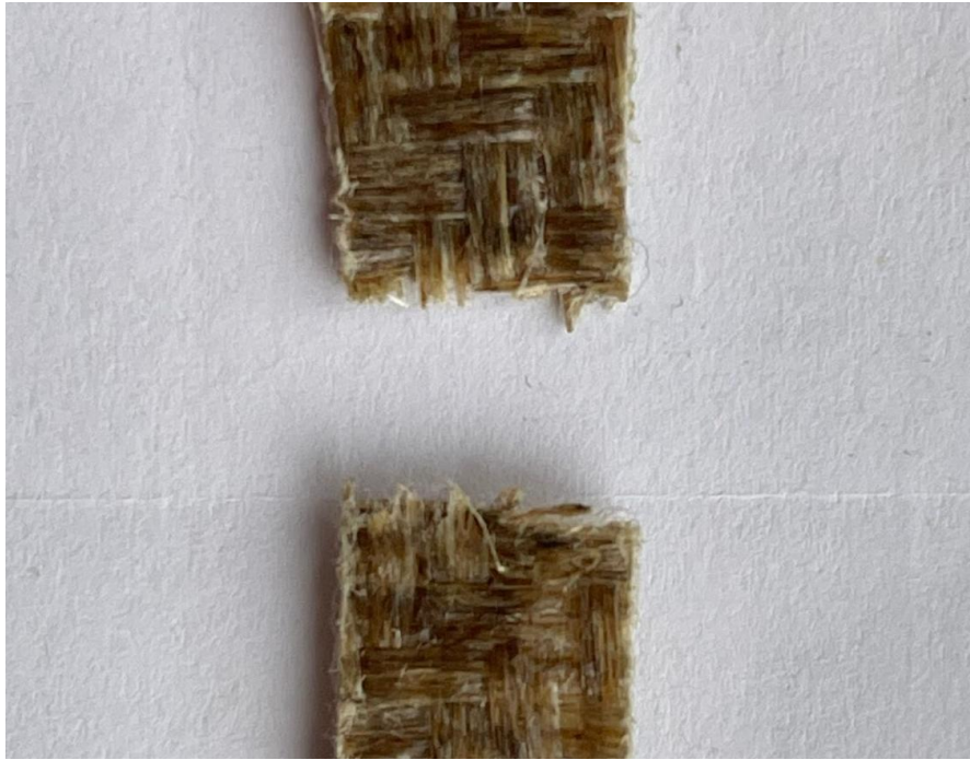
Figure 5 - Macro image showing the brittle tensile failure in specimen 1
