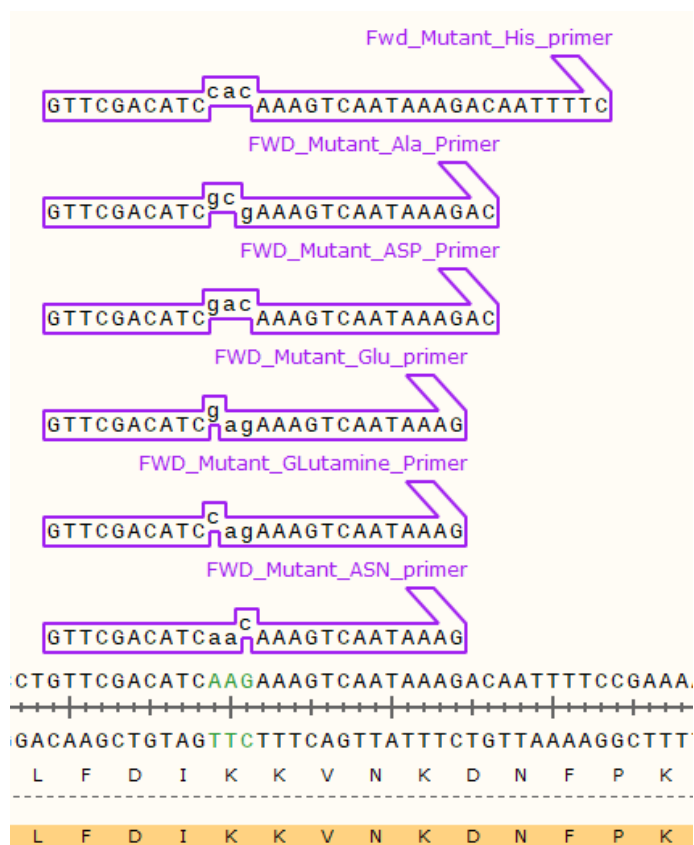
Figure 29: Map of the plasmid that was used to help design the primers that would generate the amplicon with the gene that gives a mutant protein when it undergoes transcription/translation. (top) Shows the sequence where the primers were made to bind to, the green highlight sequence of the top strand shows the codon for the 115-lysine residue above shows how the primer sequence was altered that would give a different codon for another amino acid. (bottom)
