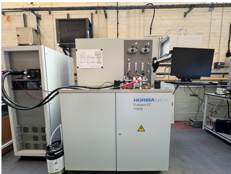
Figure 3.12 Image of the HoribaFuelCon testing system.
