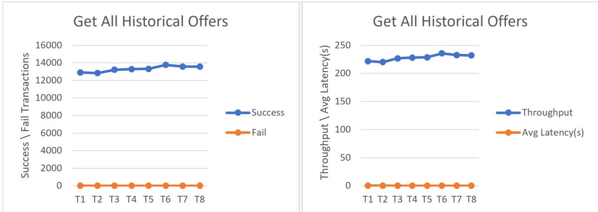
Figure 6.8: Success and fail transactions rates (left side). Throughput and average latency (right side) of "GetAllHistoricalOffer" smart contract.
