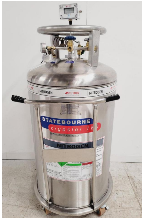
Figure 3.11: Cryostor 180 Liters liquid nitrogen dewar
