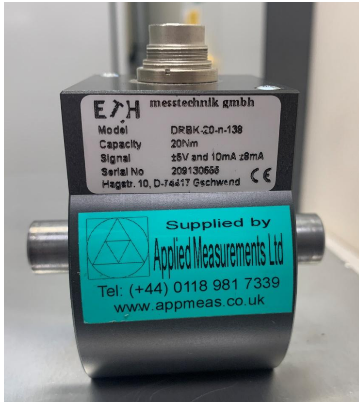
Figure 3.19: Applied measurements DRBK torque and rotational speed sensor
