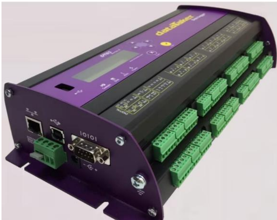
Figure 3.13: DataTaker DT85 data acquisition device
