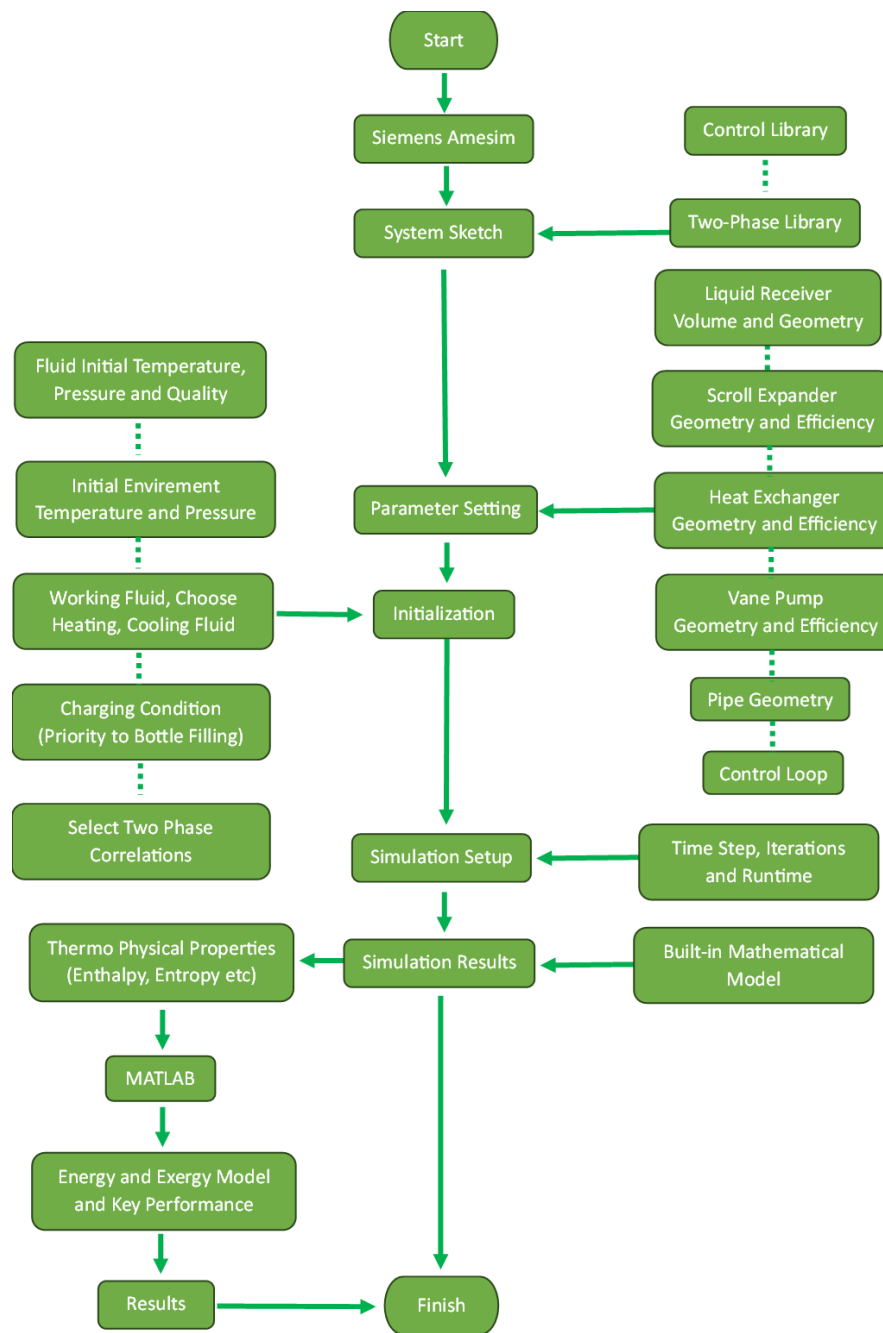
Figure 4.1: Flowchart of the dynamic numerical model methodology
