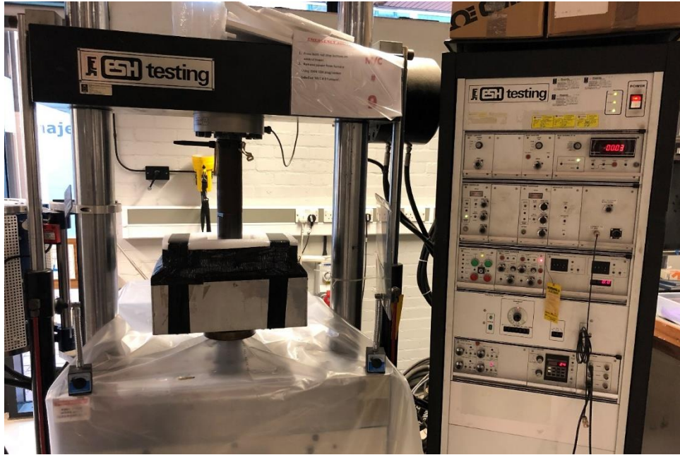
Figure 3.14 The ESH hydraulic testing machine set-up for test at -196^{\circ}\text{C} .
