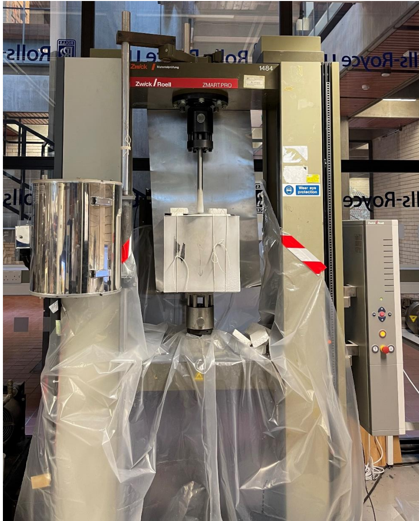
Figure 3.4 Tensile testing set-up for tests carried out at -196 °C.
