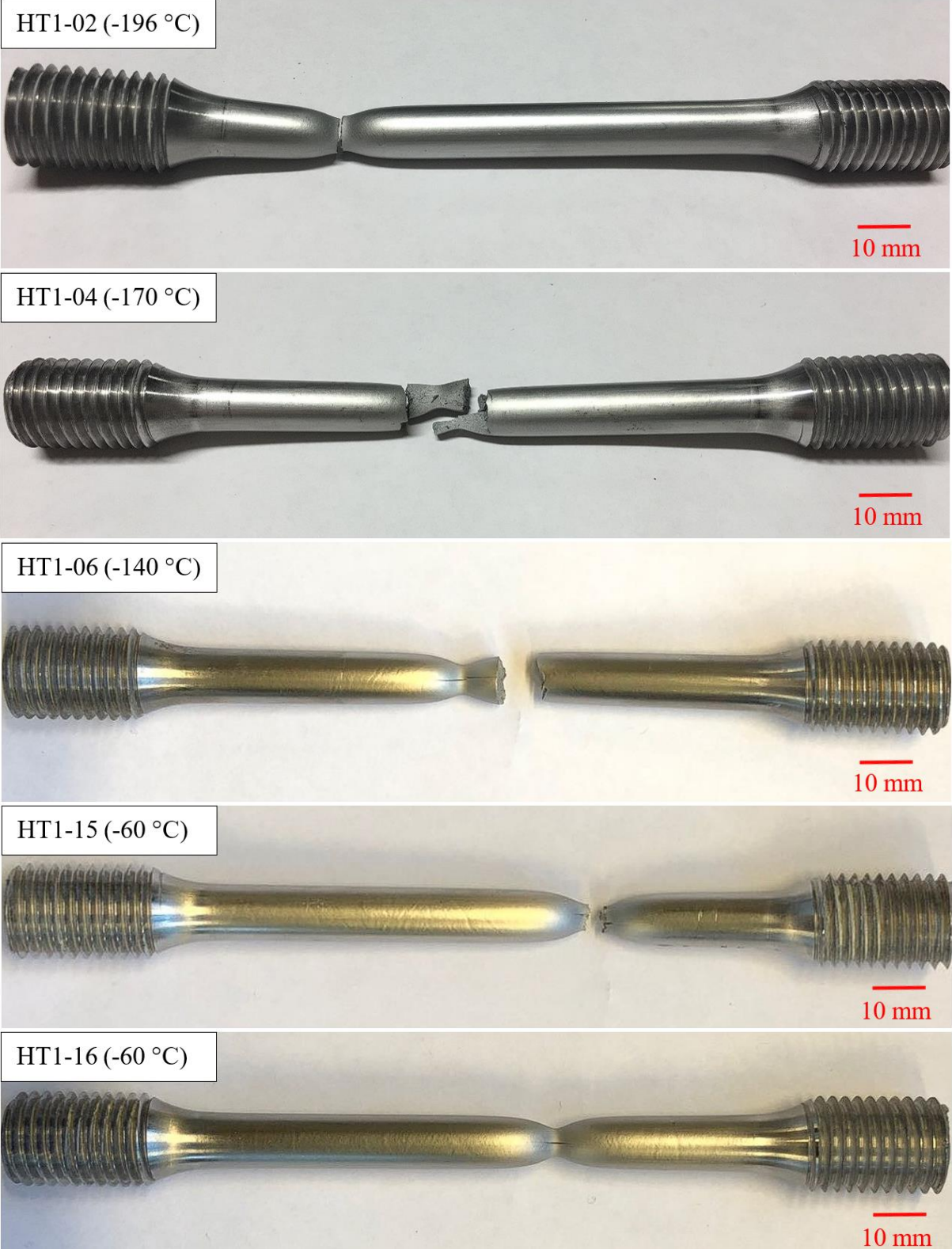
Figure 4.9 Fracture profiles of HT1 and HT2 specimens at different temperatures, (a) HT1 and (b) HT2.
