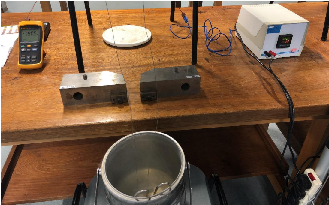
Figure 3.8 Set-up for the development of the temperature-time curves.
