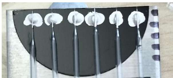
Figure 5.6: Photograph of nanopipettes mounted on an aluminium plate, with carbon adhesive pads, silver paste bridging the nanopipette tip, and 5 nm carbon coating.
