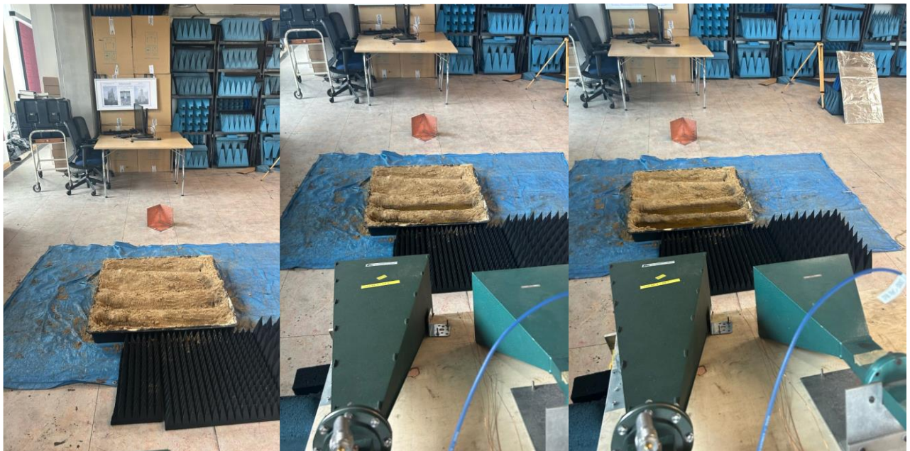
Figure 5.56: Varied applications of oil (0L to 9L) on 14 cm rough surface profile
