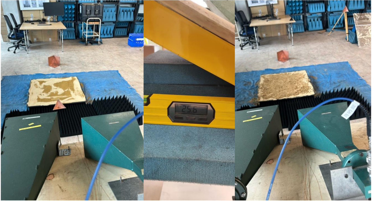
Figure 5.43: Experimental setup for a flat sand profile
