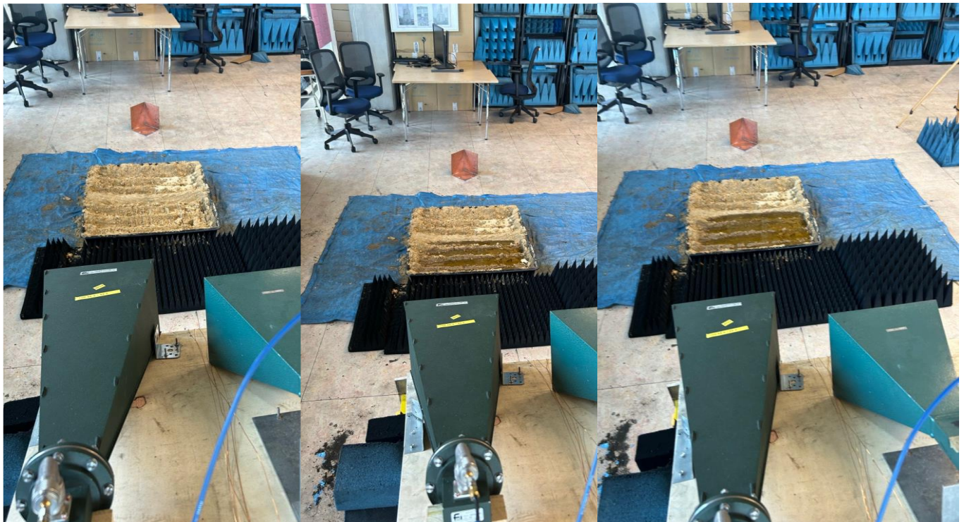
Figure 5.53: Varied applications of oil (0L to 9L) on 7 cm rough surface profile
