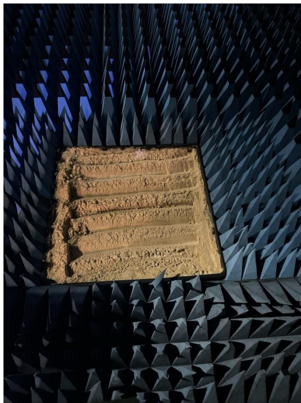
Figure 5.34: Dry sand rough surface profile with 7 cm surface roughness
