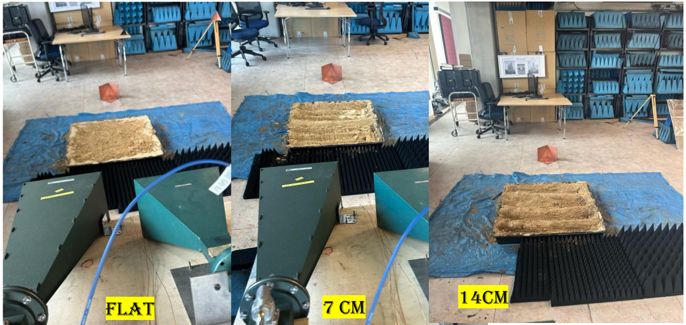
Figure 5.50: Dry Flat sand profile as well as 7cm & 14cm rough surface profiles
