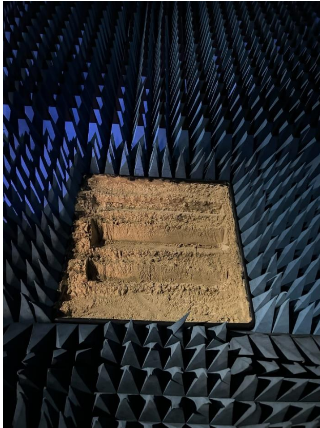
Figure 5.35: Dry sand rough surface profile with 14 cm surface roughness
