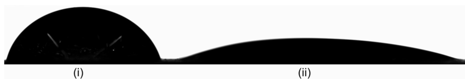
Figure 5.14. Water droplets on SHS-ZnO after the (i) 3-hour and (ii) 24-hour immersion in bacterial culture medium with contact angles being 61.5 \pm 3.7^\circ and 19.7 \pm 0.5^\circ respectively.
