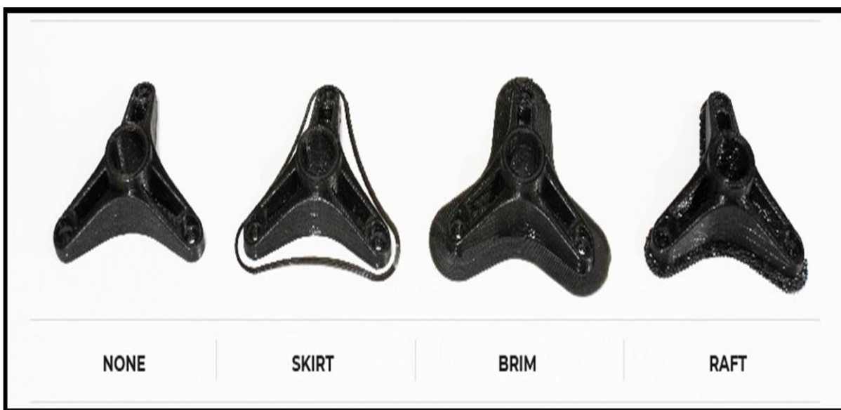
Figure 5.7: Different types of adhesion support used in FDM 3D printing.
