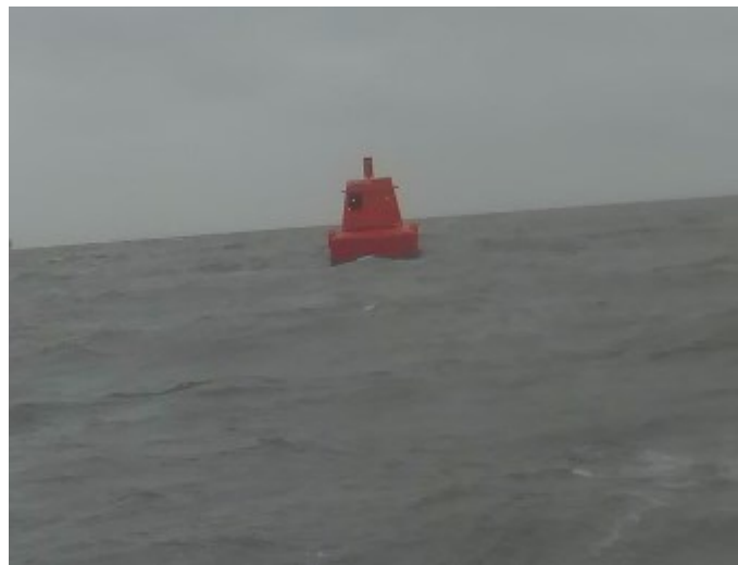
Figure 6.2-4 The Peel Wreck Buoy, around 25 m from the radar. The size of the buoy was around 3.5 m tall and a 3 m diameter. The top of the buoy was likely deliberately shaped to form a corner reflector so that it would show as a bright reflector on the radars of passing ships.
