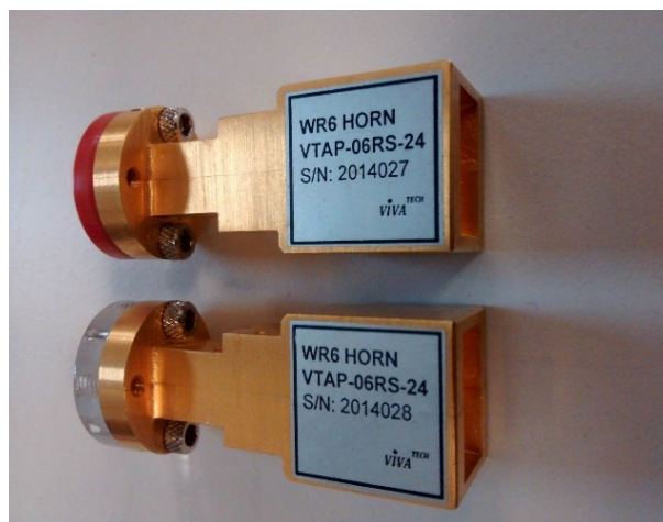
Figure 5.5-1 10-degree pyramidal horns for 150 GHz radar – flanges at left, apertures at right. Approximately 6 cm in length.
