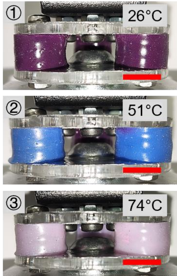
Figure 3.41 Photographs of the thermochromic elastomer-encapsulated FMHE compensator at different temperatures.
