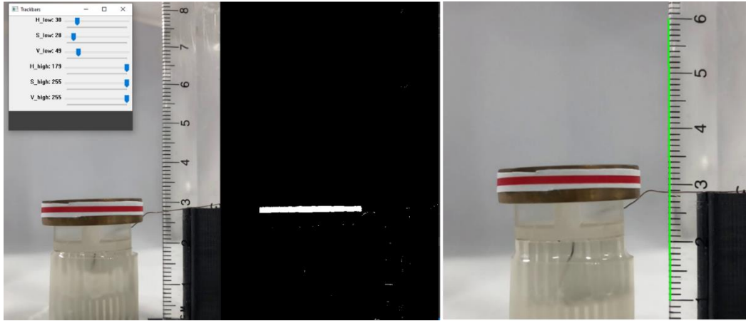
Figure 4.60 Mask (left) and measurement line (right) for tracking of CLMM movement.
