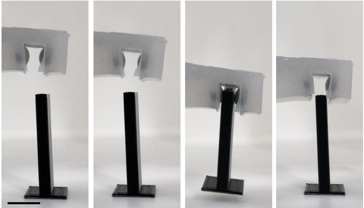
Figure 4.73 A soft robotic gripper inflated and deflated by CLMM picking up and putting down an object.
