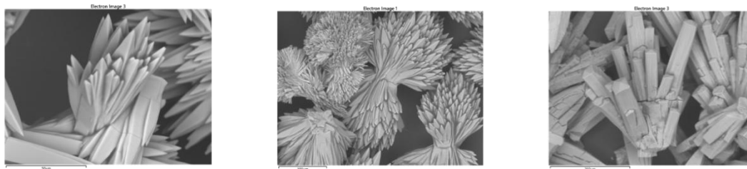
Figure 2.22: SEM images of Yb 2 (DNNDI) 3 MOF crystals at different magnifications (50 μm, 100 μm, 250 μm)
