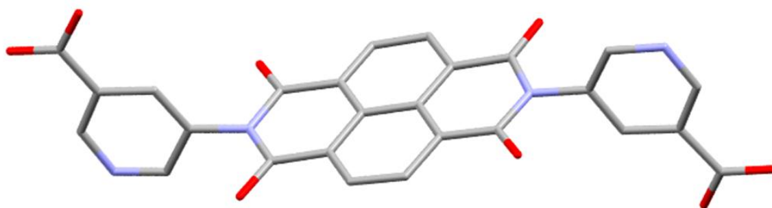
Figure 2.1: View of the single crystal structure of DNNDI. Carbon - grey; Oxygen – red; nitrogen – blue
