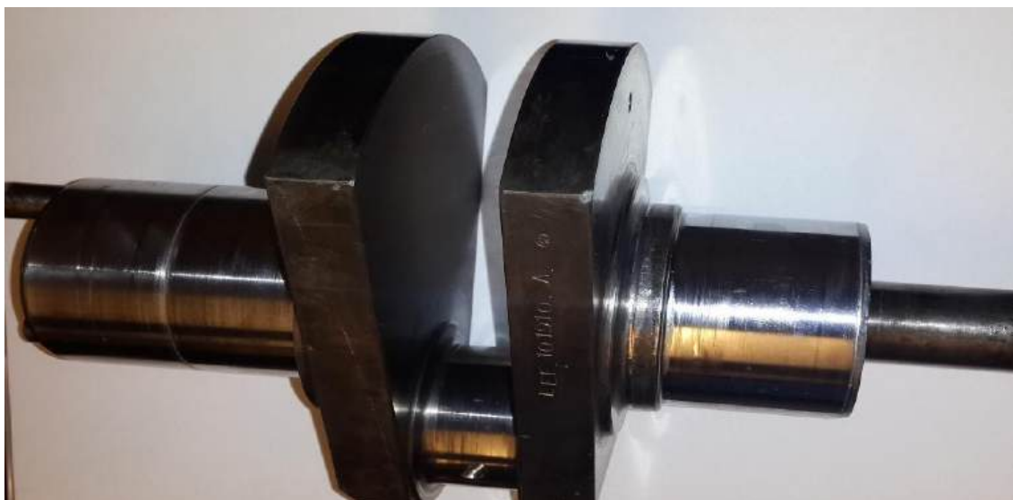
Figure 3.9 Nitrides Crankshaft for the Single cylinder Medusa thermal engine.
