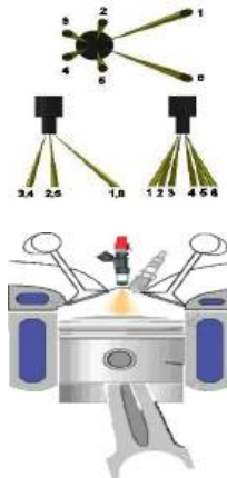
Figure 3.5 Layout of the orientation of injector spray plume and combustion systems.
