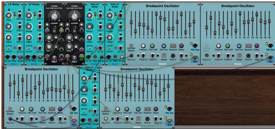
Fig. 10 – The breakpoint oscillator in a patch, producing slowly moving cluster sounds with varying timbers.
