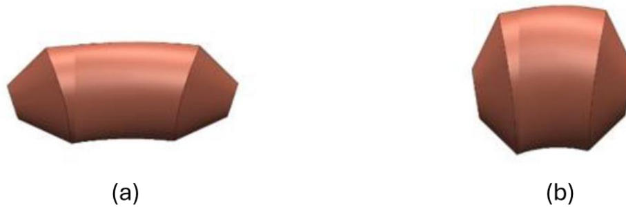
Figure 1.7 Two possible shape of the UoB combustor
