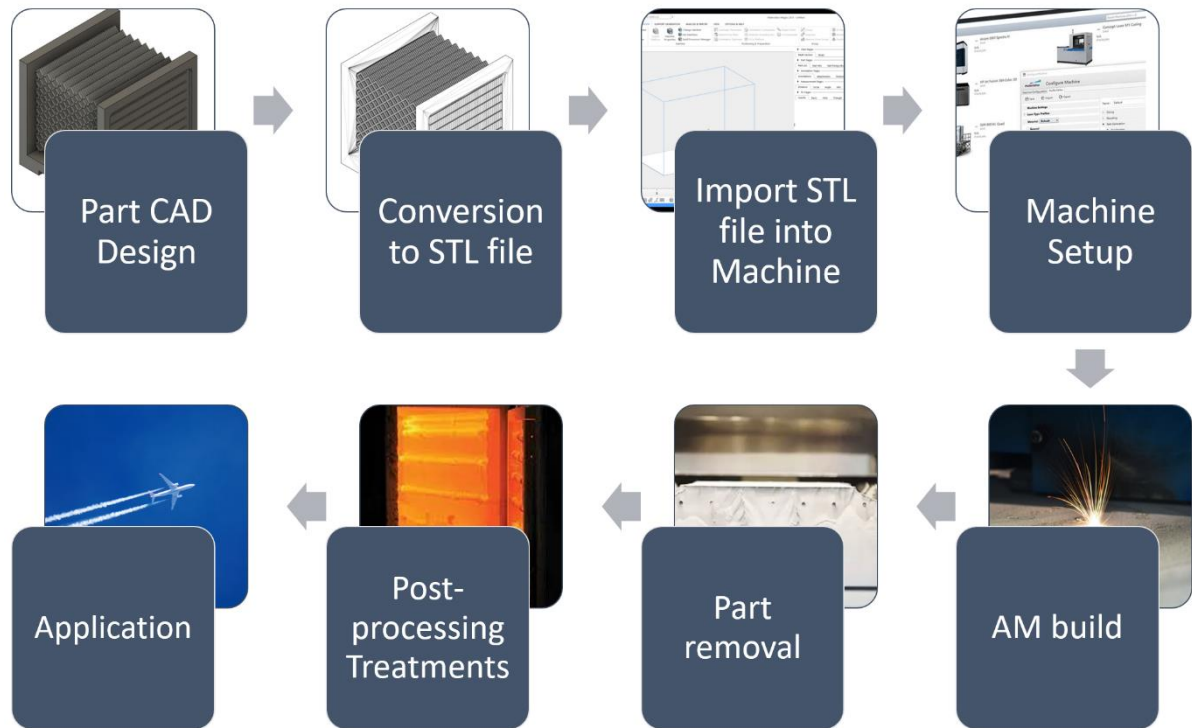
Figure 1.1. Typical flowchart of AM manufacturing steps included in production strategy.
