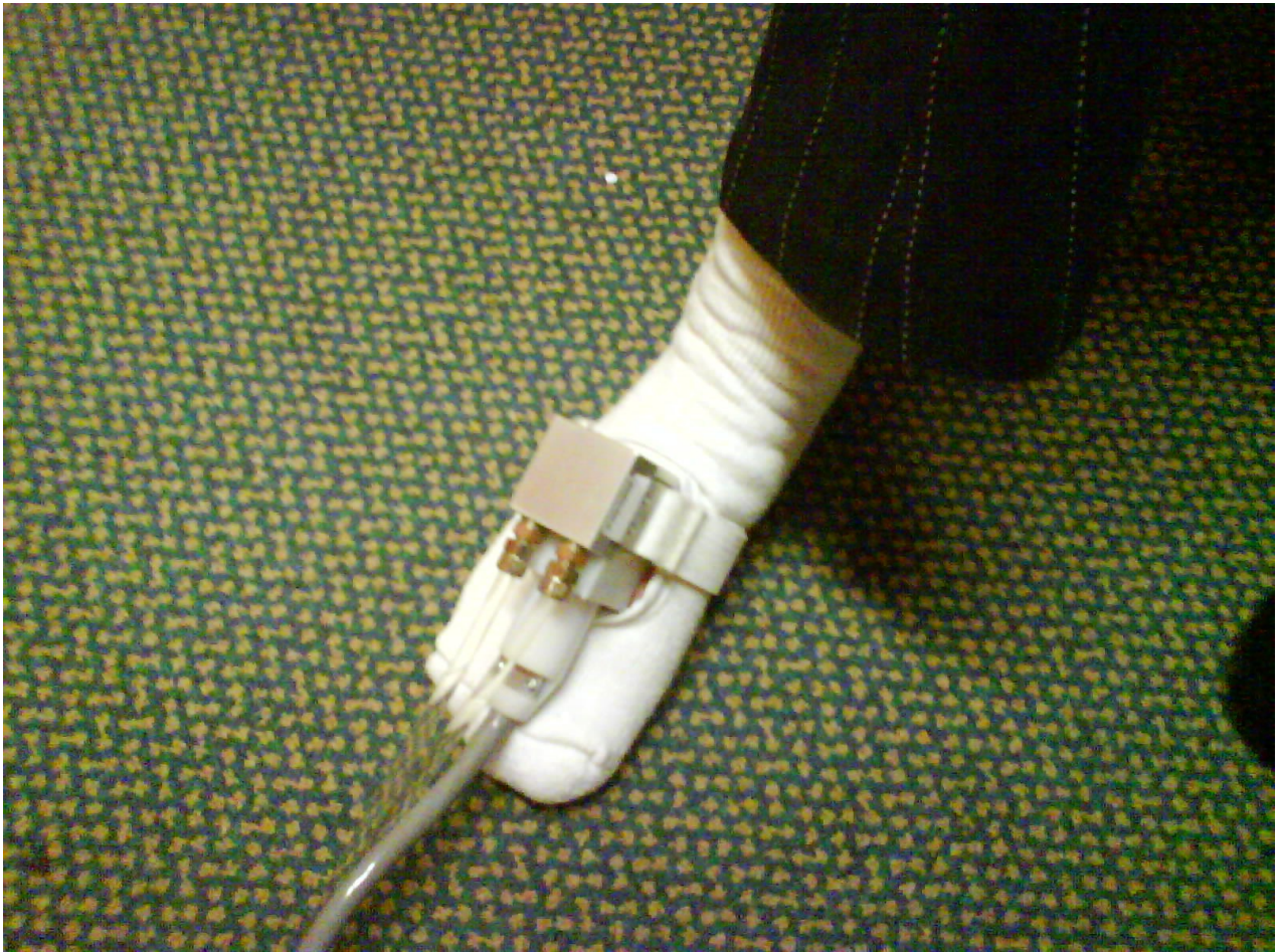
Figure 5. Measurement of Thermal and Heat-Pain Thresholds in the Right Foot. Participants wore a sock with a hole in its dorsal surface. The thermal stimulator was strapped onto the dorsal surface of the foot, through the hole, so that all four corners of the stimulator were in contact with the skin.
