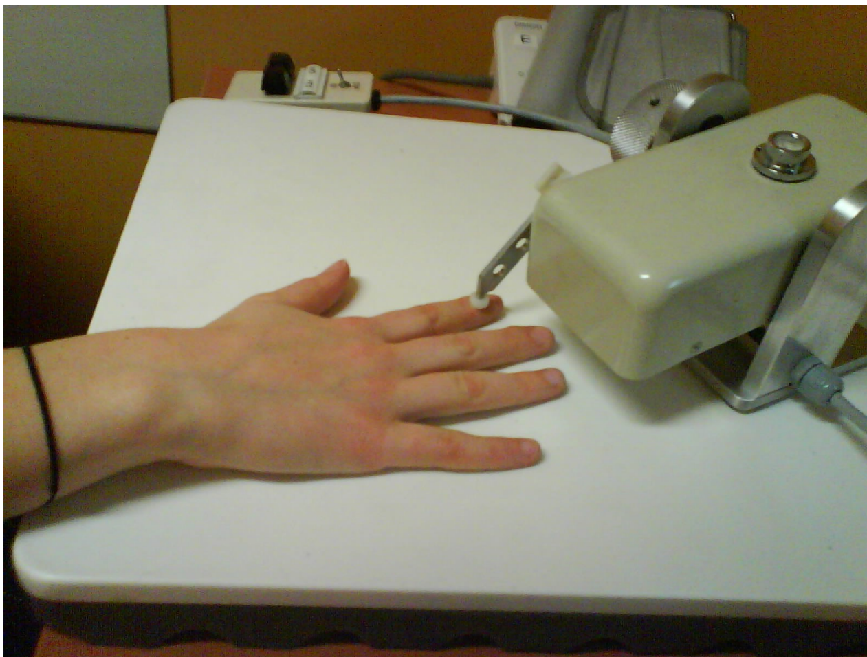
Figure 4. Measurement of Vibration Threshold in the Right Hand. The right hand rested on the vibration board and the vibration stimulator was placed on the index finger, in the midline between the base of the nail and the most distal knuckle.
