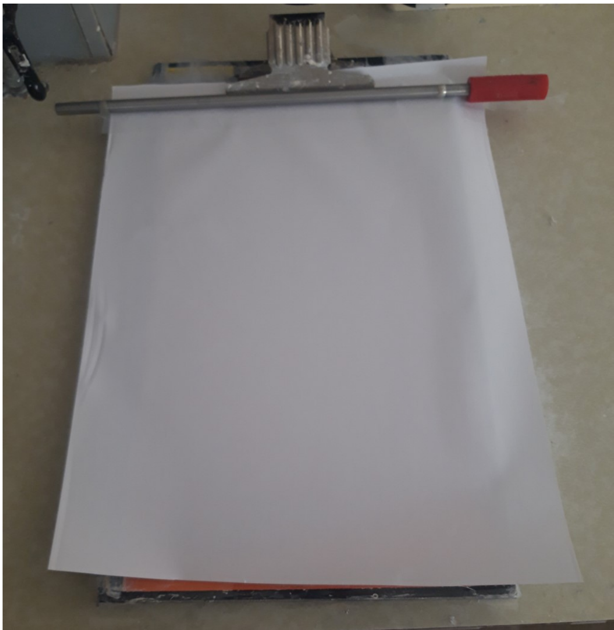
Fig. 3.1. Experimental set up for coating paper with MFC using the manual laboratory rod coating method.
