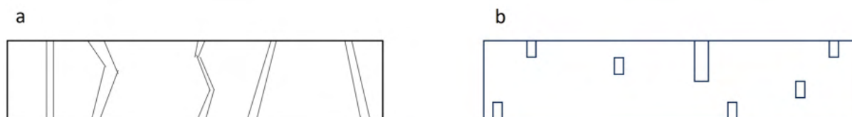
Fig. 5.36. Schematic diagram showing how increasing cellulose fibrillation may lead to improved barrier properties due to a lower volume of connecting pore space.
