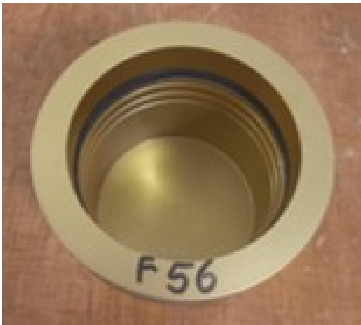
Fig. 3.9. Example of a permeability pot used to measure WVTR. Film or paper sample is screwed into place between rubber gaskets above an empty chamber.
