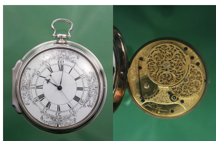
Figure 2.6: Image of H4 chronometer developed by Harrison [52]
