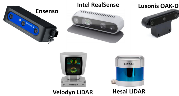
Figure 1.2: Different depth camera and LiDAR devices used in industries for 3D perception.
