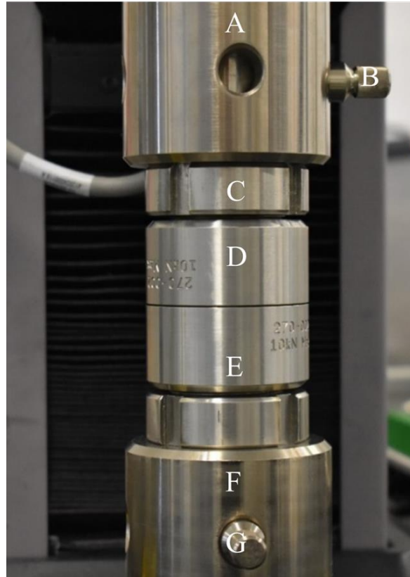
Figure 3.18 Arrangement for determining the machine compliance: compression loading of flat platens. ( A and F ) standard Clevis adaptors (has female inside). ( B and G ) Clevis pin (male). ( C ) universal grip joint. ( D and E ) Bionex stainless steel compression platens [89].
