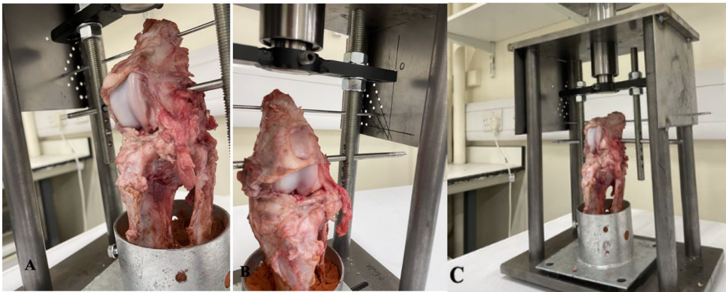
Figure 46. Specimen mounted at different flexion angles (A) 30° (B) 45° (C) 90°.
