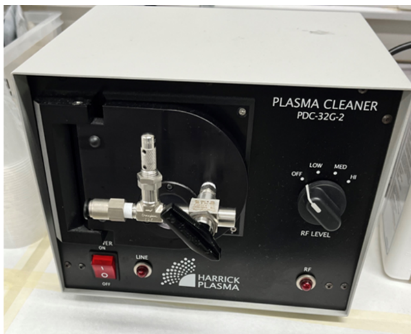
Figure 2.4: Harrick Plasma Cleaner is used to clean the surface of wafers for use as substrates.
