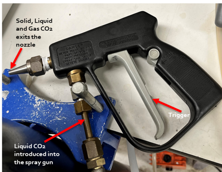
Figure 2.3: An in-house-designed spray carbon dioxide system for snow jet cleaning.
