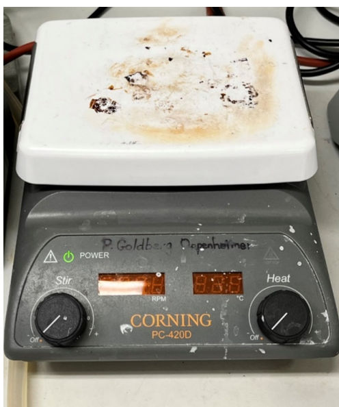
Figure 2.8: The hotplate was used during the softbake process to improve photoresist adhesion to the surface and for the post-exposure bake process for cross-linking when the negative photoresists were used.
