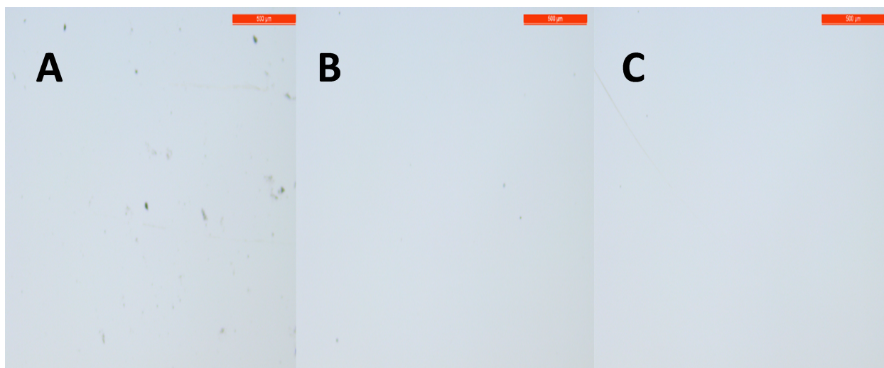
Figure 2.2: It shows the optical microscope images of silicon wafers before cleaning (A), after cleaning with solvents and a plasma cleaner (B) and using cleanroom wipes and the snow jet cleaning process (C). The scale bar is 500 \mu\text{m} .
