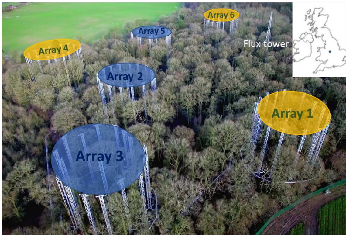
Figure 3.1: Schematic of the BIFoR-FACE site from (Hart et al., 2020). Fumigated arrays are represented in orange and ambient arrays are in blue.
