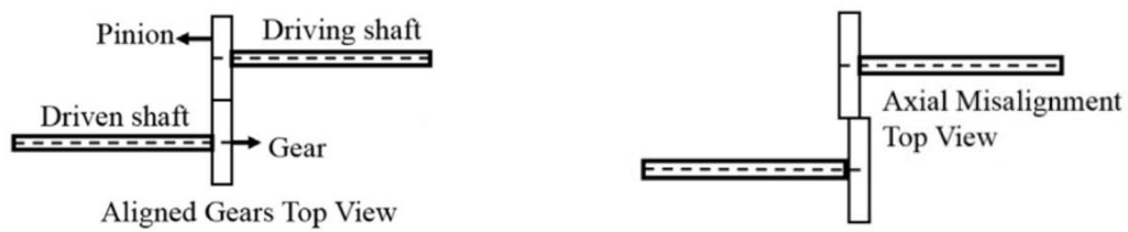
Figure 2. 6 Pinion and Gear Axial Misalignment Errors (after, [9])
