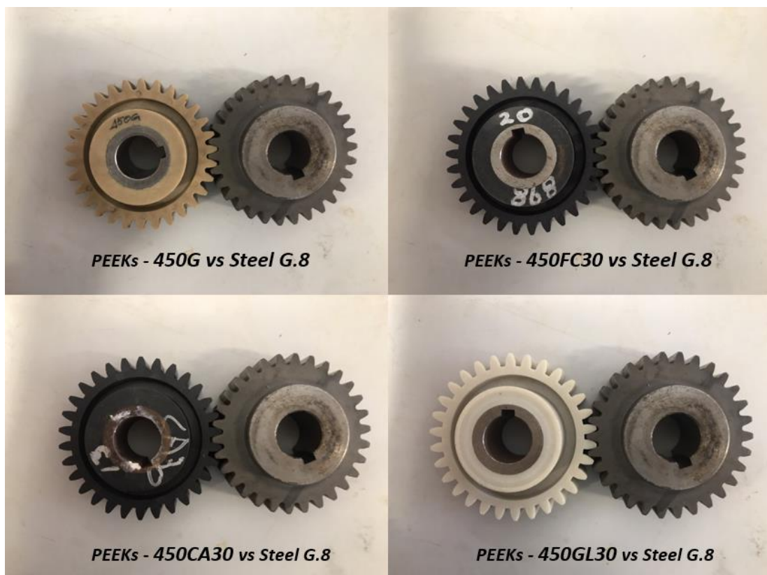
Figure 4. 5 Meshing Display of 450G, 450CA30, 450FC30, and 450GL30 vs STEEL Grade 8
