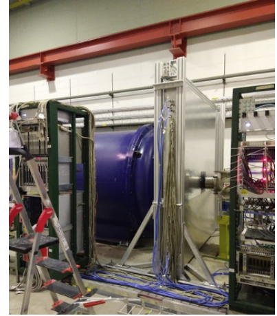
Figure 4.2: Left: A schematic of the ANTI-0 detector showing the support frame, central sheet and counters. Note the horizontal line just below the mid-point of the detector delimiting the top and bottom parts. [101] Right: Picture of the ANTI-0 as installed in TCC8, with the blue decay vessel to the left and beam pipe to the right. [107]
