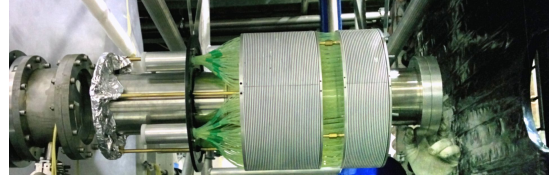
(b) IRC installed on the K12 beam line.
