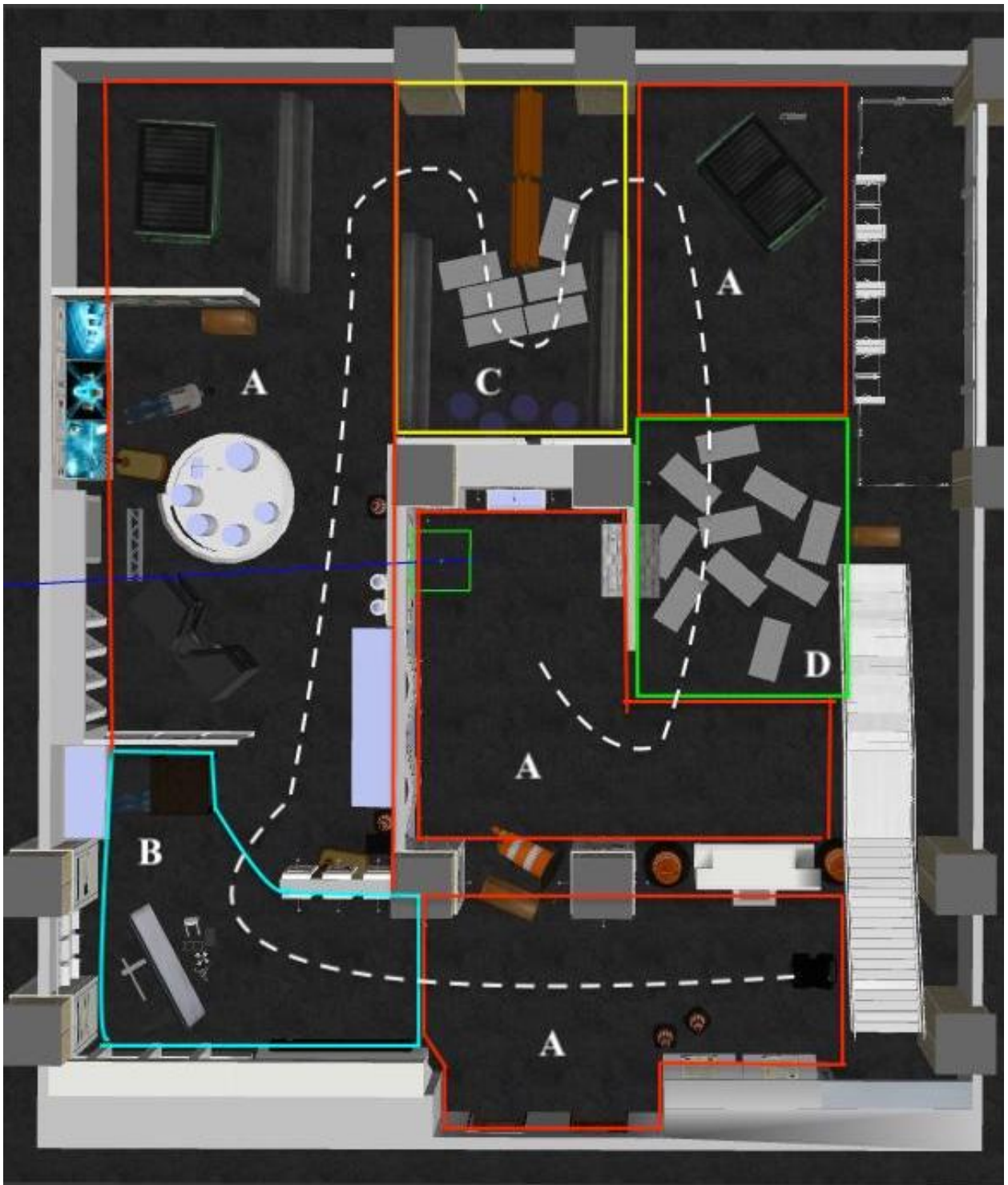
Figure 4.13: The tessellations (A to D) and the feasible robot path plan P (dotted line) for the navigation task
