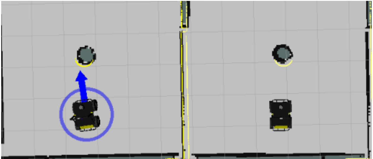
Figure 5.8: Active Robot Marker Visual Cue: The robot on the left is currently active, and is in manual control
