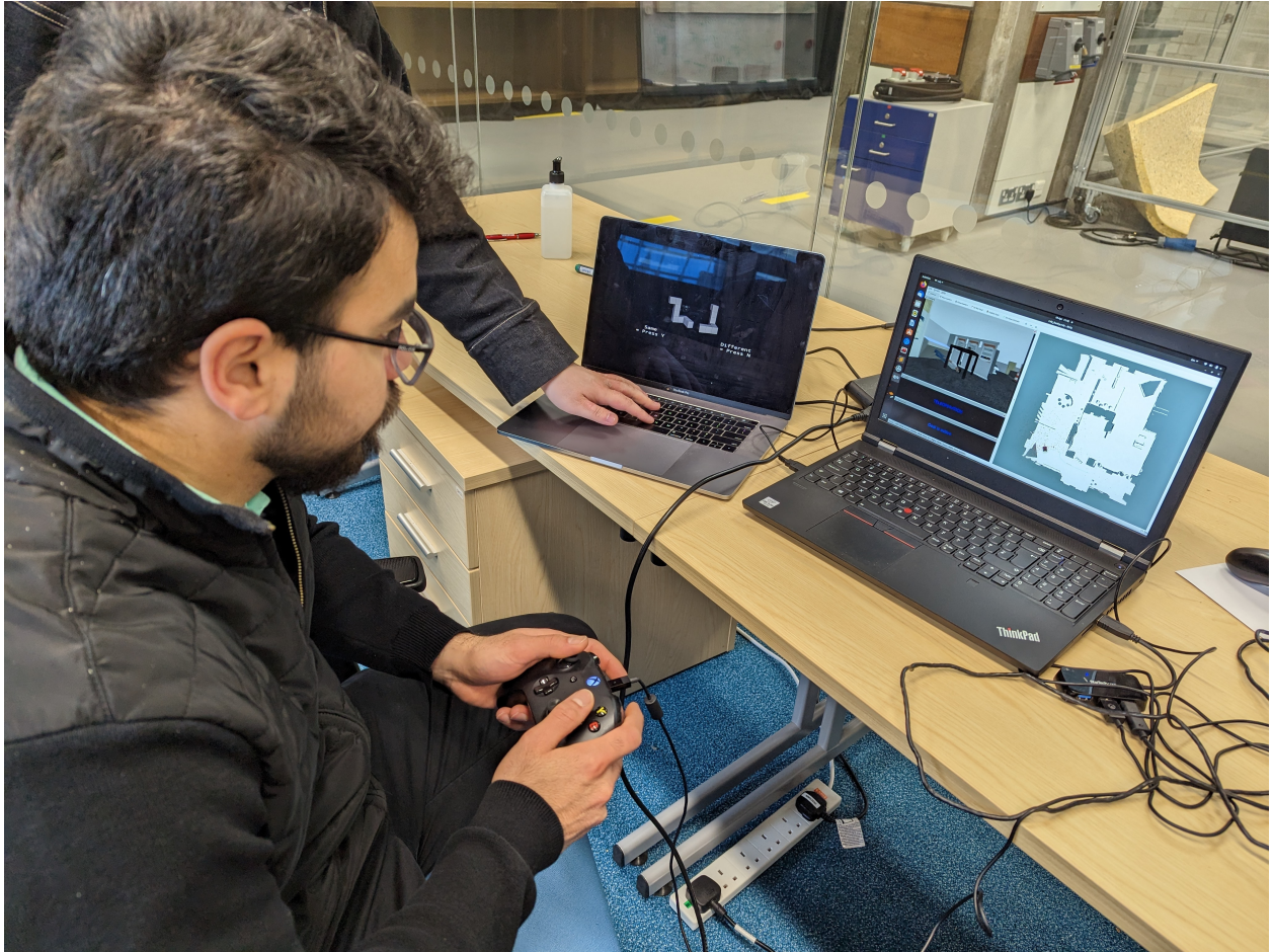
Figure 4.16: The control unit used for the experiment. The participant controls the robot using a joystick and views it on the screen. The secondary task is shown on another laptop, and is monitored by the experimenter
