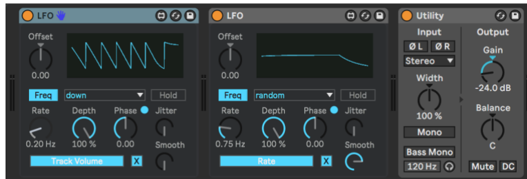
Figure 30 - Two low-frequency oscillators controlling the volume level of the audio track containing the thirteen club recordings for Sounds of Clubbing , resulting in quick level change bursts.
