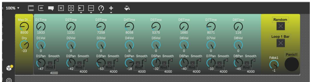
Figure 8 - Custom designed multiple delay line effect in Max for Live for Sounds of Echoes .
