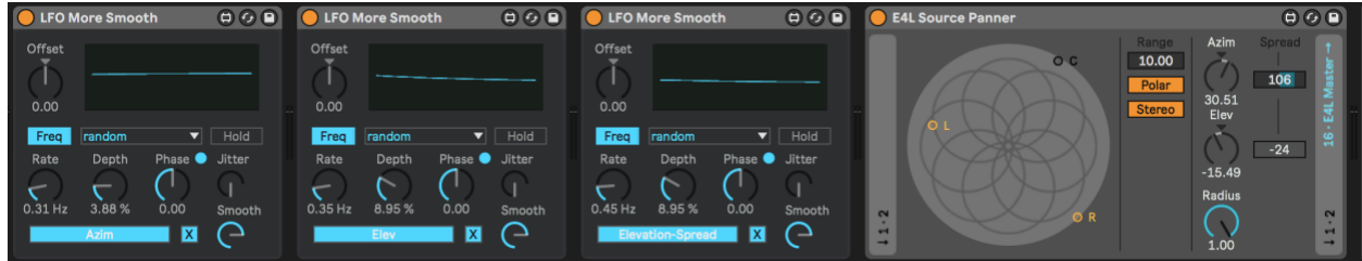
Figure 37 - Low-frequency band information modulated by low-frequency oscillator controlling binaural panner parameters for Sounds of Synthesizers .
