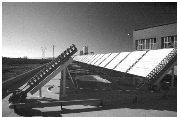
Figure 1.17: One of the first pilot plants for photocatalysis, employing a slurry reactor (in a static concentrator array) installed at latitude 40^\circ (Arganda del Rey, Madrid, Spain). Costing estimates in Table 1.1 for plant scale PCs are taken from this plant's operation[63]. Reproduced with permission from Malato et al. [69].
