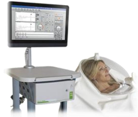
Figure 2.2: Picture of the Moxus metabolic cart for indirect calorimetry. Picture on the left is the MOXUS metabolic cart showing the O 2 and CO 2 analysers, gas cylinders, mixing box, canopy, and the associated laptop and software for data acquisition and analysis. Picture on the right showing an example of a participant's positioning under the canopy.
