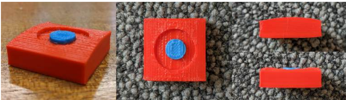
Figure 6.26: 10 mm diameter (height 2 mm) cylindrical print (blue) in situ printed onto the curved bottom surface of the circular recess (20 mm diameter, depth 2 mm) in the top face of the 3D printed base (red) (30 × 30 × 10 mm with top surface radius of curvature 57 mm). The top surface of the base, the bottom of the recess, and the top surface of the surface addition print have the same curvature.
