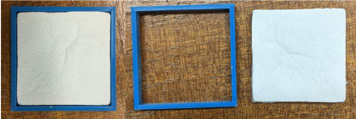
Figure 6.31: From left to right: The clay alignment base before removal from the mould, the empty mould, the cured clay alignment base.
