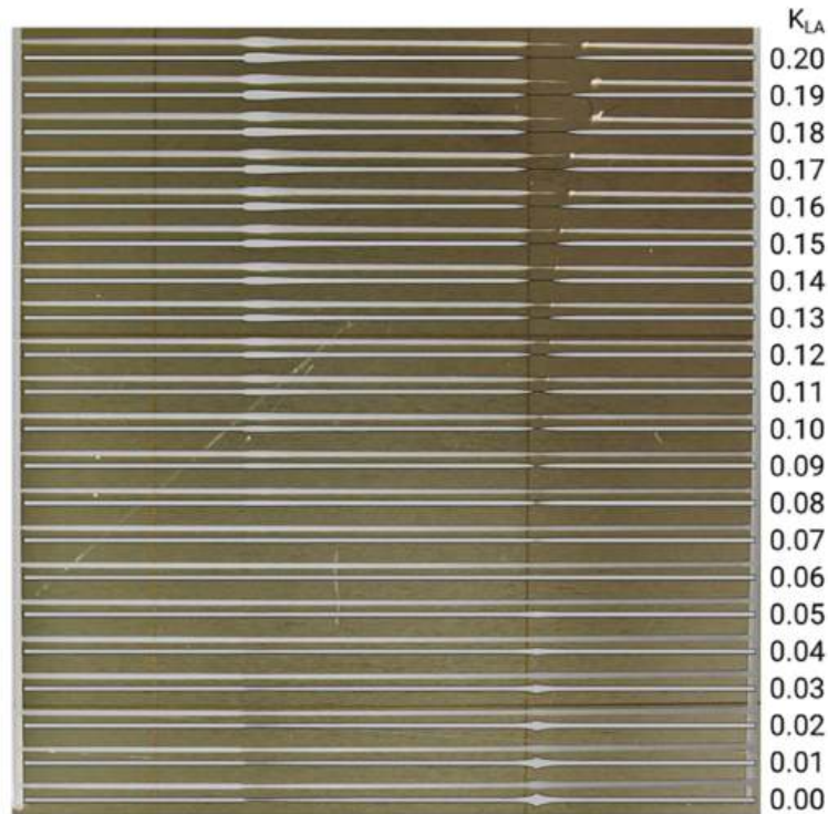
Figure 4.18: Experimental results of PLA filament deposition with Marlin Firmware Linear Advance Calibration [138].
