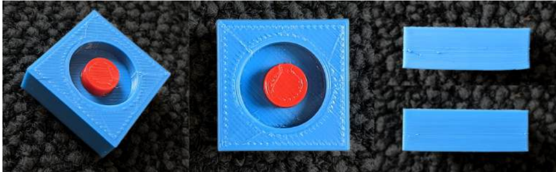
Figure 6.22: 10 mm diameter ( height 4 mm) cylindrical print (red) in situ printed onto the bottom surface of the circular recess (depth 4 mm) in the top face of the 3D printed base (blue) (30 × 30 × 10 mm). The top surface of the implant is in line with the top surface of the base.
