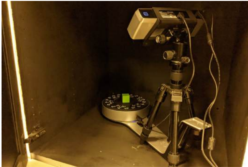
Figure 4.2: A 3D printed cube on the coded turntable of the scanner inside the darkbox.
