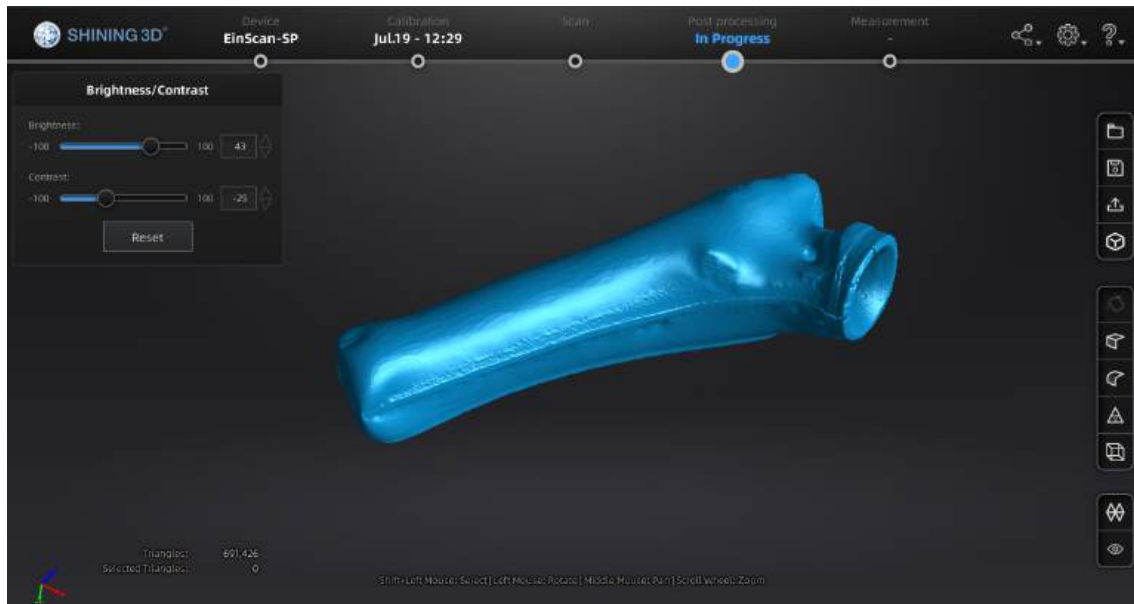
Figure 3.2: Screenshot of the Shining3D software-generated watertight medium detail mesh of the bone model section
