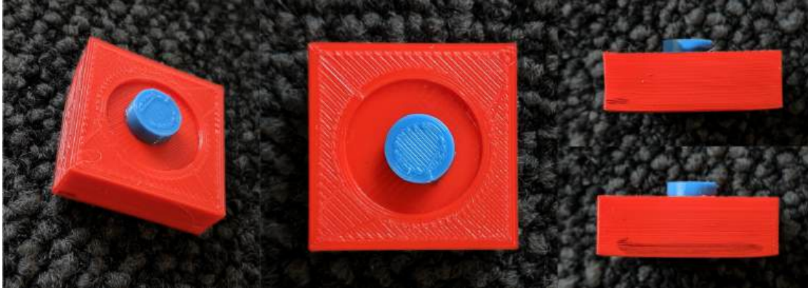
Figure 6.20: Second print of the 10 mm diameter (height 4 mm) cylindrical print (blue) in situ printed onto the bottom surface of the circular recess (depth 1 mm) in the top face of the 3D printed base (red) (30 x 30 x 10 mm). The surface addition print is more central.
