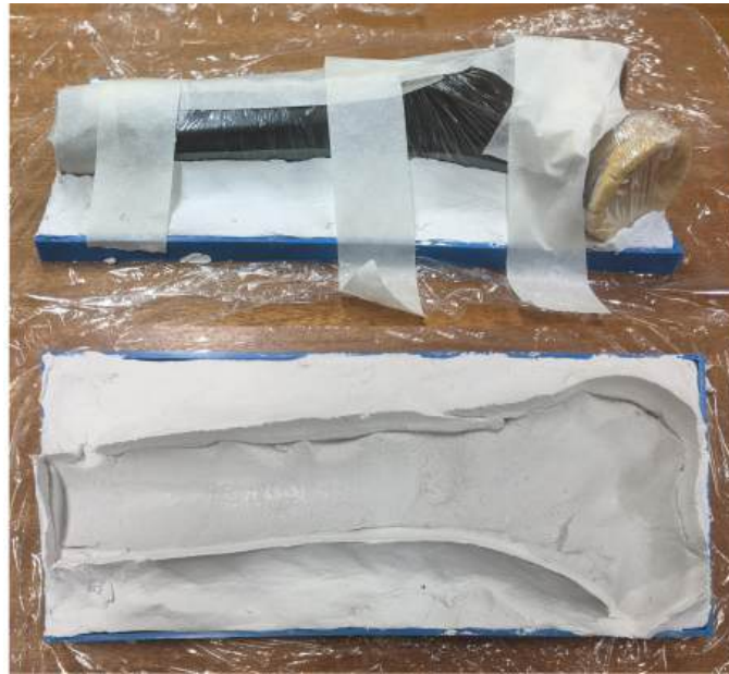
Figure 6.47: Creation of the holding mould for the Sawbone bone model. Top: The bone model secured in the mould during curing. Bottom: The empty holding mould during the curing time.
