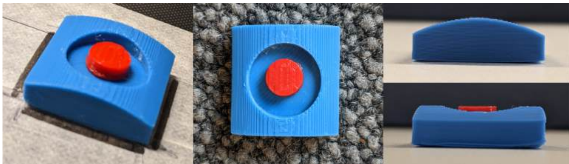
Figure 6.24: 10 mm diameter (maximum height 4 mm) cylindrical print (red) in situ printed onto the bottom surface of the circular recess (20 mm diameter, maximum depth 4 mm) in the top face of the 3D printed base (blue) (30 x 30 x 10 mm with top surface radius of curvature 30 mm). The top surface of the base and of the surface addition print have the same curvature.
