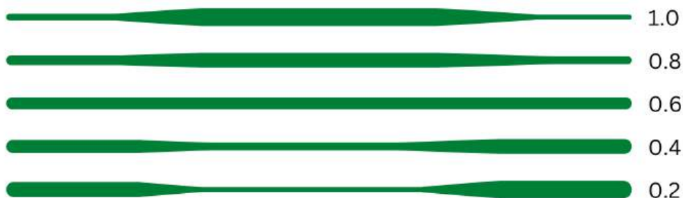
Figure 4.17: Simplified model of Linear Advance Calibration effects on filament deposition; example K-values for PLA and the effect on filament deposition as viewed from above.
