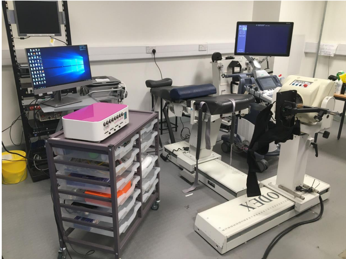
Figure 5. Experimental setup used in our study. On the right side, Biodex isokinetic dynamometer can be seen.
