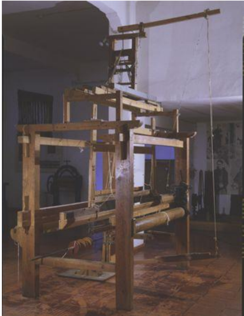
Fig. 2.38, Unknown author. Jacquard loom, 1920, Museu Nacional do Traje e da Moda, Portugal. Wood, 410 cm (height), 172 cm (width), 281 cm (length). Includes a device that moves the punched cards. © Museu Nacional do Traje / DGPC, all rights reserved.
