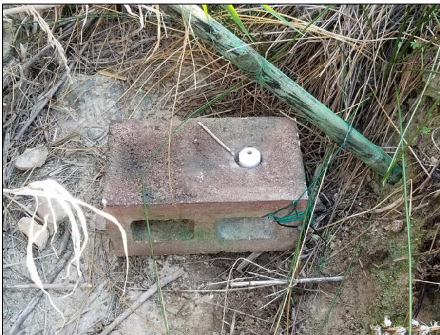
Figure 3.2. Onset HOBO U20L-04 with HOBO U2X Protective Housing deployed at Wied ta' Miġra l-Ferġa case study site.
